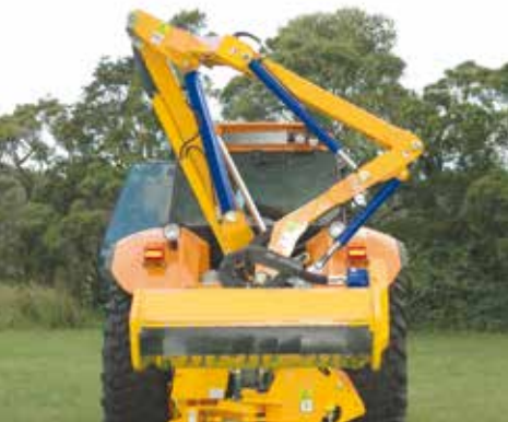
Transport position Folding 3rd arm allows compact transport position.
